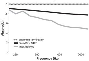
NRC of anechoic termination 1.00 NRC of fabric in front of anechoic termination 0.85
